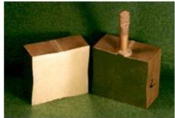
To illustrate the effectiveness of the HIP process a 25mm diameter hole was machined in two halves of a stainless steel block 75mm square. The edges of the block were welded together, the air evacuated from the hole and the evacuation pipe sealed to create a subsurface pore. The block was HIPped and subsequently cut in half to reveal fully dense material and complete absence of any pore.
