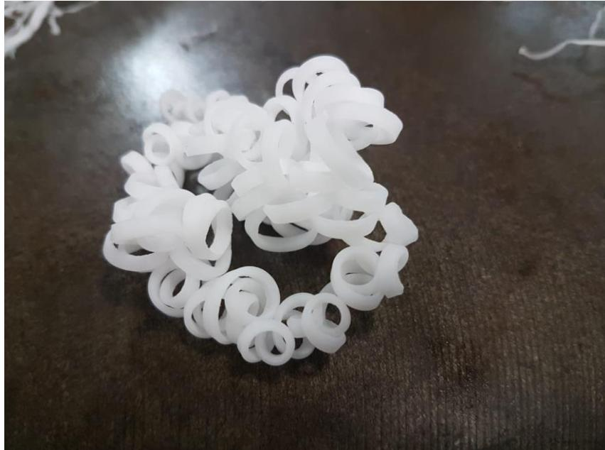
*(Rosçamento;  $V_c = 250\text{m/min}$ ;  $F = 2\text{mm/rot}$ ;  $A_p = 1,25\text{mm}$ )*
